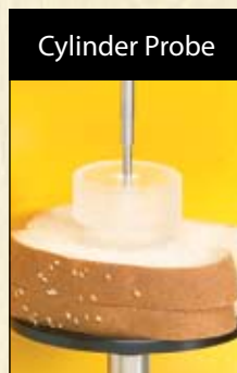
A cylinder probe can provide uniform compression over fixed surface area. Ideal for most bakery items and more.
