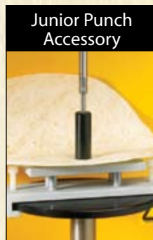
Puncture compression test for solid materials such as tortilla wraps and films.
