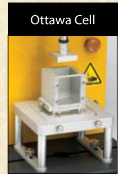
Compress and extrude samples with a travelling plunger. Ideal for dry cereal, small fruits and vegetables and more.
